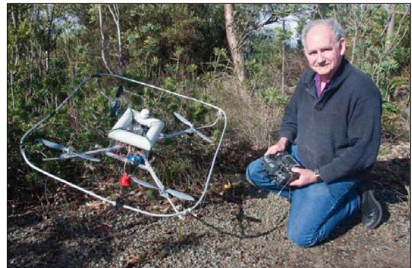
John Moore shows a prototype of the HerbiCopter remote controlled spraying unit.
