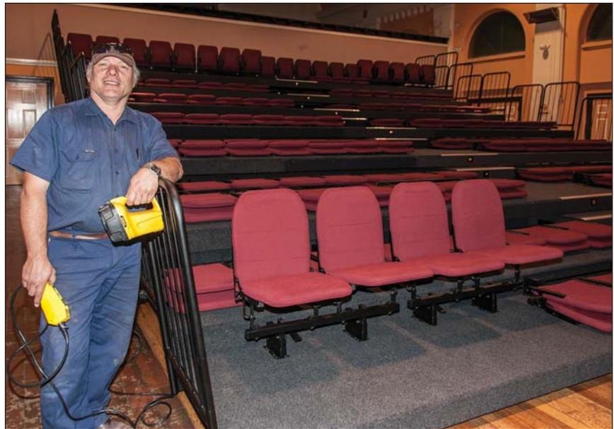
*Building maintenance officer Don Cumby rolled out 213 tiered seats in about a minute. Each bank of seats folds flat so the multiple levels can roll back for compact storage.*
